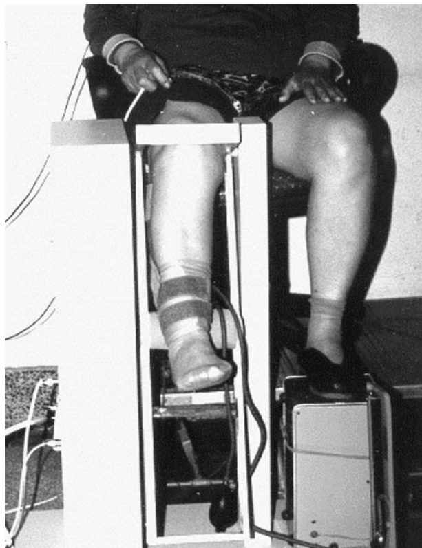
Figure 2 Customised apparatus used to test passive motion sense of the knee joint.
